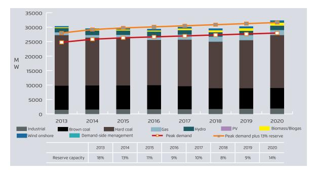
Fig. 1a Power balance on the National Electricity System up to 2020, not taking into account the cold reserve.
